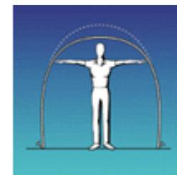
If the sides are pushed out, the top is flattened slightly and the dome shape is restored.
